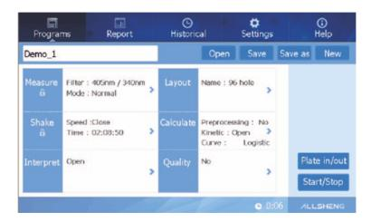
AMR-100 keep with high visual and logical user interface of software, it can be offered a comprehensive inbuilt calculations, such as blank subtraction, quantitative curve fit, quantitative classification and kinetic calculations, as well as the versatile reporting tool and make data reduction.
